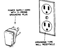
If the circuit does not have a grounding type receptacle, it is the responsibility and obligation of the customer to change the existing receptacle to a properly grounded receptacle in accordance with the National Electrical Code and applicable local codes and ordinances. The third ground prong should not, under any circumstances, be cut or removed.
