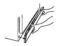
To remove the defrost pan, grasp the base grille at both ends and pull it straight out. Slide the pan out from underneath the cabinet.
